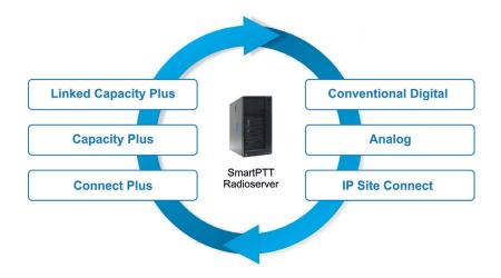
Routing rules are easily created using the dispatcher console. Routes can be one-way, two-way, between different networks and radioservers. Typical routes include:
